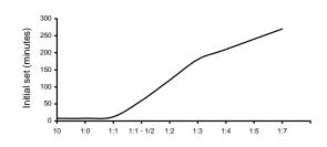
Mortar: 1:1w/c 0.35Temperature:  $+21^{\circ}$ C
